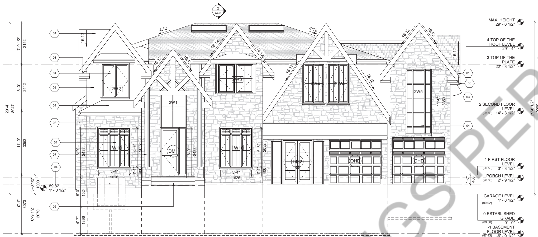
2 SOUTH ELEVATION (Front) A3.0 1/4" = 1'-0"
